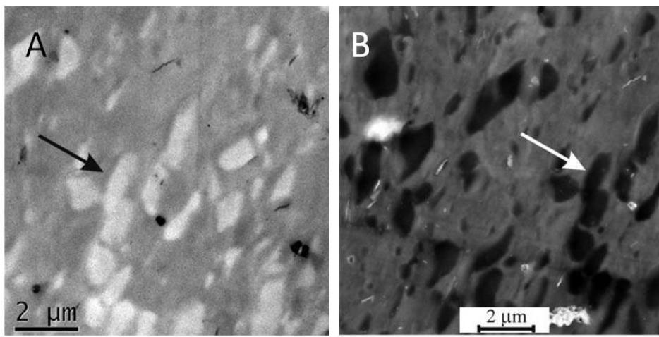
A thermoplastic vulcanized (TPV) unstained specimen imaged in different modes: (A) bright field conventional TEM image (approximately in focus); (B) high-angle annular dark field (HAADF) scanning TEM image of the same area as imaged in A (arrows indicate same specimen features).
